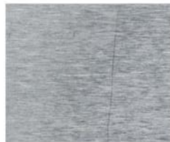
Surface finish: fine-machined, and grinded, Ra 0.4 μm
