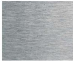
Surface finish: machined, Ra 0.8 μm
