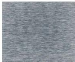
Surface finish: fine-machined, and grinded, Ra 0.2 μm
