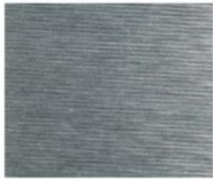
Surface finish: machined, Ra 1.2 μm
